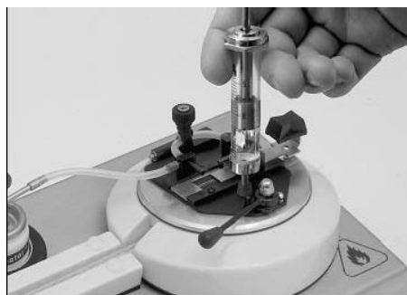
2. Inject 2 ml or 4 ml sample material into the sample cup. Wait one or two minutes for vapor equilibrium to occur.
