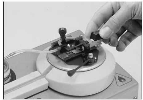
3. Introduce test flame - observe flash or no flash.
